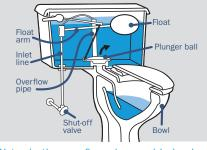
Water in the overflow pipe could also be caused by a pinhole in the float or a worn washer on the inlet line.
